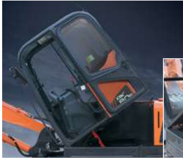
Tilting cabin for easy maintenance
