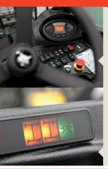
FNR on Joystick puts maximum control at your fingertips. Select the driving direction at the touch of a button, while still keeping a grip on both the steering wheel and the joystick for improved safety and productivity.
