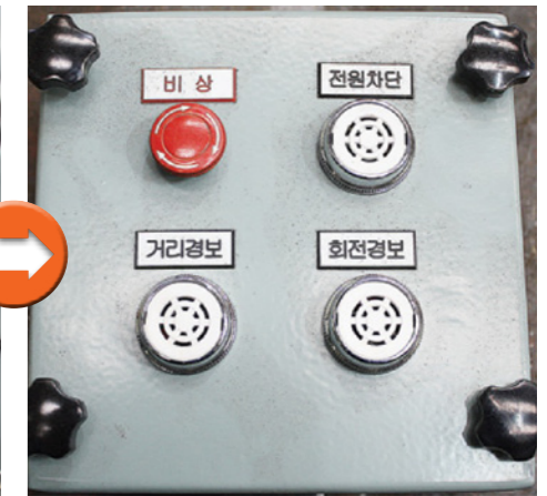
Excavator controller Displays warning information and emergency power shutoff
