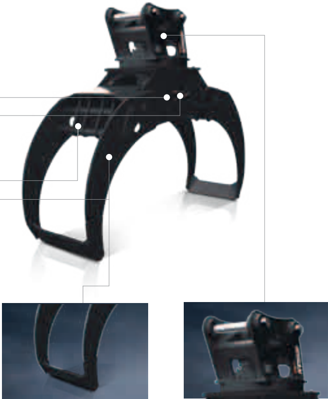
Optimized jaw shape for holding small object
