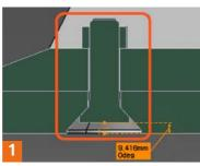
PLOW BOLT FOR CHANGEABLE PARTS New plow bolt will be applied on tooth adaptor and cutting edge
